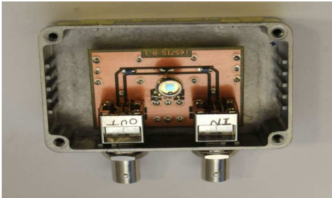
PPA PCB Circuit 1/2 (photodiode detector with tune circuits)
