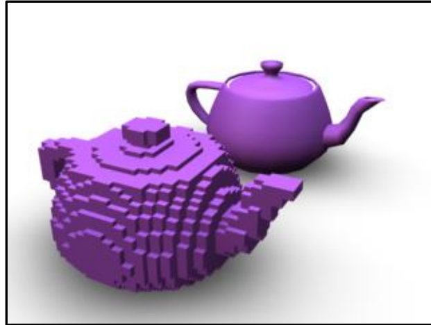
Figure 2.5: Voxel representation of a smooth teapot as on the right (Source: Mattausch, O., 2011*)
