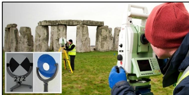
Figure 4.13: Scanning Stonehenge using 'butterfly-shape' and sphere shape target (Source: Greenhatch Group, Ltd., 2010*)
