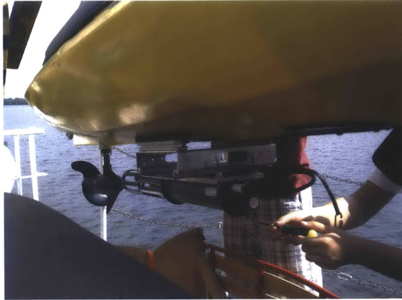
Figure 1-2: Image of a SCOUT kayak equipped with a YSI multi-parameter sonde.
