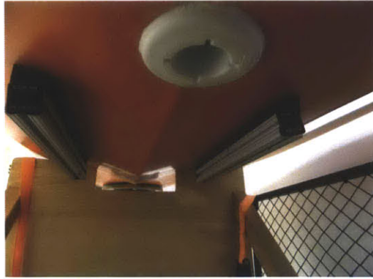
Figure 2-6: Image of instrument mounting channels on the underside of a SCOUT kayak.
