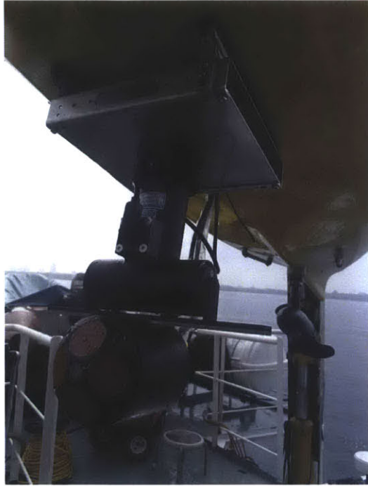
Figure 2-7: Reorienting ADCP assembly mounted underneath a SCOUT kayak.
