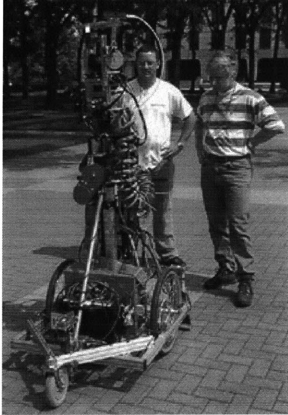
Figure 1.4: The Argus pose-camera platform estimates its location and orientation while acquiring images.
