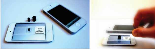
Figure 2. Prototype microscope. A sample is rear-illuminated, in this case using a secondary cellphone display, and photographed using a cellphone camera. Optical magnification is achieved by mounting a small lenslet at its focal length to the sample.
