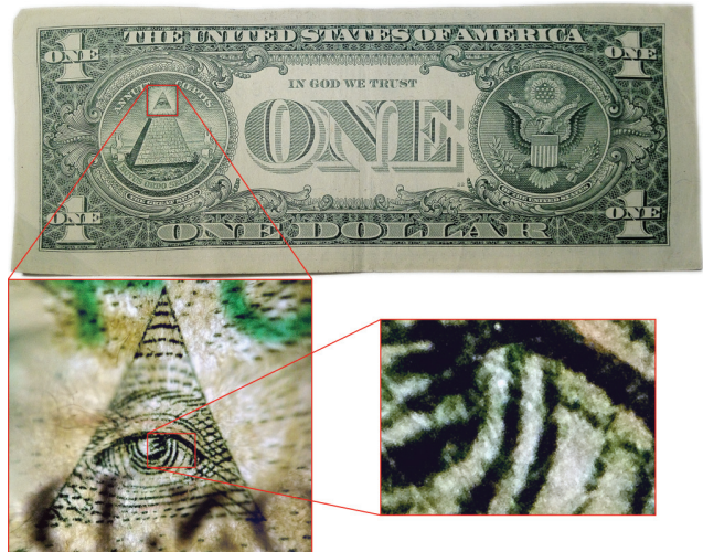
Figure 5. Panoramic imaging. While each photograph of our setup only covers a limited field of view, our unique optical setup allows us to combine multiple photographs into a wide field of view panorama as seen on the lower left. Due to the rear-illumination, the text on the other side of the bill is also visible in the panorama.
