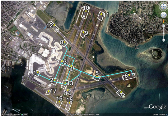
Fig. 1. Layout of the airport surface at Boston Logan. Nodes in the network model are marked with white boxes. The configuration-specific network for departures from Runway 27 has been highlighted in light blue.
