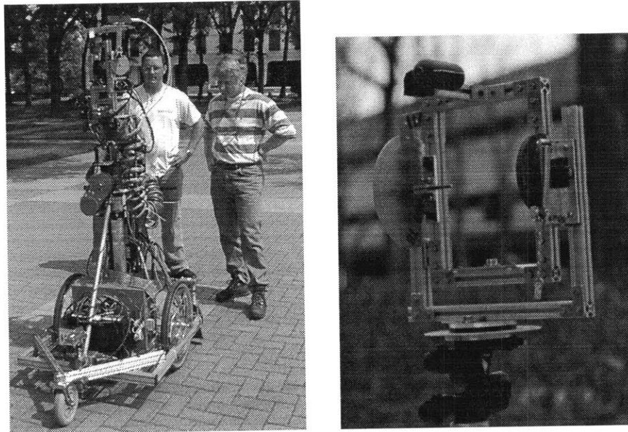
Figure 2: A view of Argus and close up of pan tilt head.
