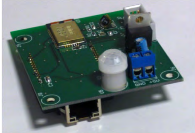
Fig. 4. Room node circuit board.
