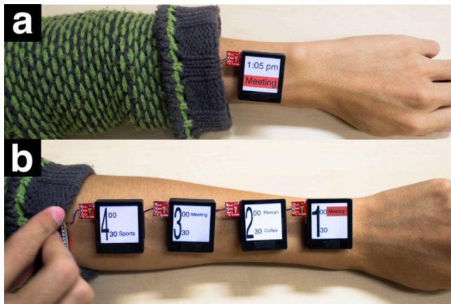
Figure 4. Using the sleeve for semantic zooming. Moving back the sleeve reveals more details about the user’s appointments.
