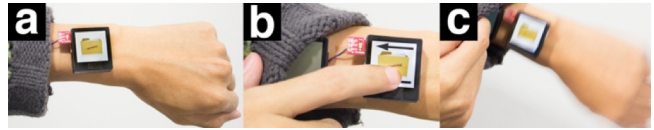
Figure 3. Using the sleeve as a container for storing items. The user can swipe-in an item into the sleeve (a, b) and bring it back by shaking the wrist while lifting the sleeve (c).
