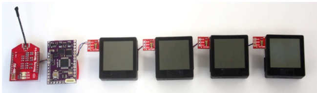
Figure 2. The hardware setup consists of four interconnect displays, each equipped with a light sensor to detect movements of the sleeve. An IMU measures the arm's orientation.
