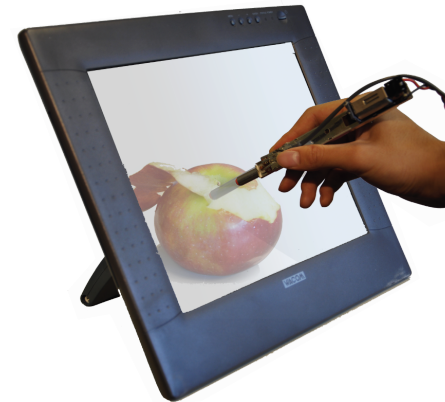
Figure 6. More portable Beyond prototype image, using camera based tracking and touch screen.
