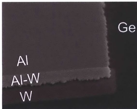
Figure 6-6: A scanning electron microscope image of an Al-W interface from CDMS II.
