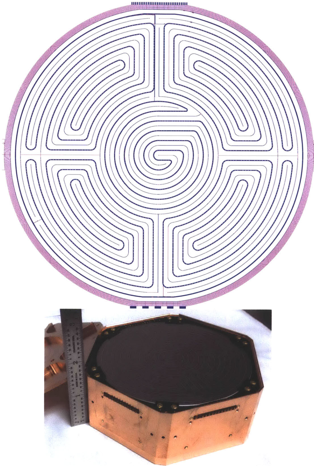
Figure 13-2: Side 1 of the iZIP6: a preliminary version of the SNOLab detector (top) and a photo of the first iZIP6 fabricated (bottom). The spacing of the TESs along the QET ribbon structures is much larger than it will be in the final SNOLAB detector, increasing the detector resistance to match the existing readout electronics.
