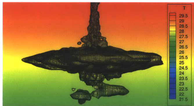
Figure 4.4 - Vertical view of the plume boundary from which the trap depth can be computed.
