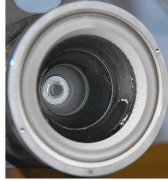
(c) The thruster after 204 [h] of operation at the conditions given in Table 2.12, for a total run time of 269 – 274 [h].
