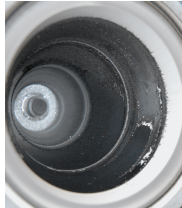
(b) Photo of the right half cone surface, facing the anode.
