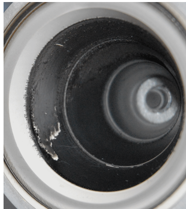
(a) Photo of the left half cone surface, facing the anode.
