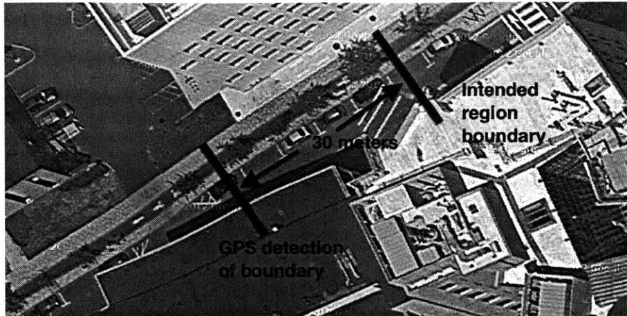
Figure 3-1: Map of programmed region boundary and detected region boundary for static GPS microexperiment.
