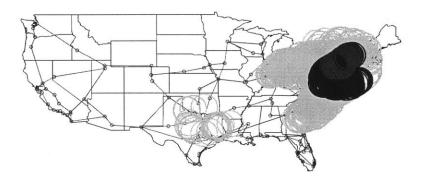
Figure 2-23: The impact of circular cuts of radius 2 on the MFST between Fort Worth and NYC. Red circles represent cuts that result in MFST = 0, black circles result in MFST = 1, and yellow circles result in MFST = 2. Cuts which intersect the nodes representing Fort Worth or NYC are not shown.
