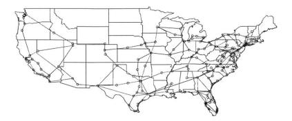
Figure 2-1: The fiber backbone operated by a major U.S. network provider [46]. Node locations are approximate and point-to-point fibers are represented by straight lines.
