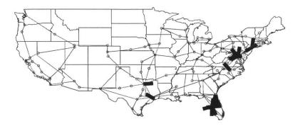
Figure 2-18: Line segments cuts optimizing TEC for h = 2 - the red cuts maximize TEC and the black segments are nearly worst-case cuts.
