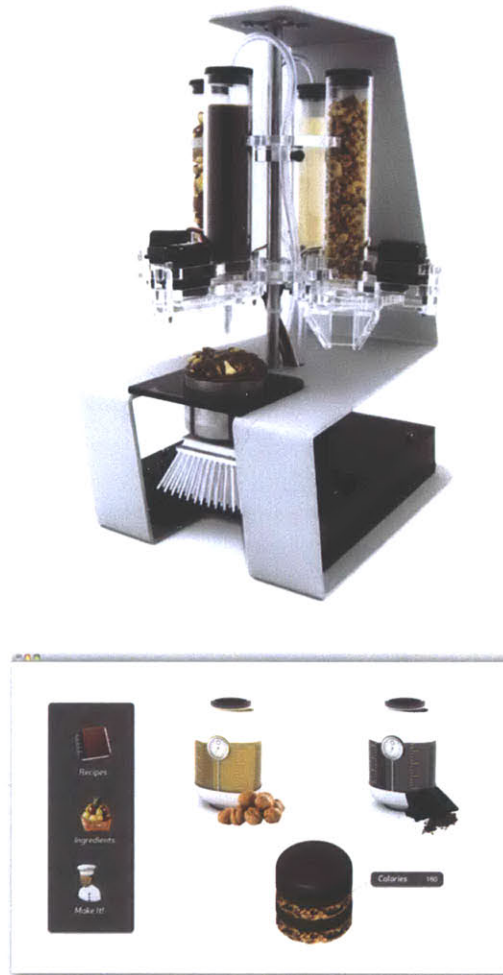
Figure 8. Digital chocolatier prototype (top) and interface that allows users to design custom chocolate candies (bottom).
