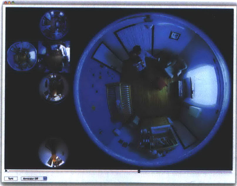
(b) TotalRecall video player, which shows 10 low resolution WINK videos and the selected full resolution SQUINT video. Here we see the child with his father in the baby bedroom, the source of the video volumes displayed in TotalRecall.
