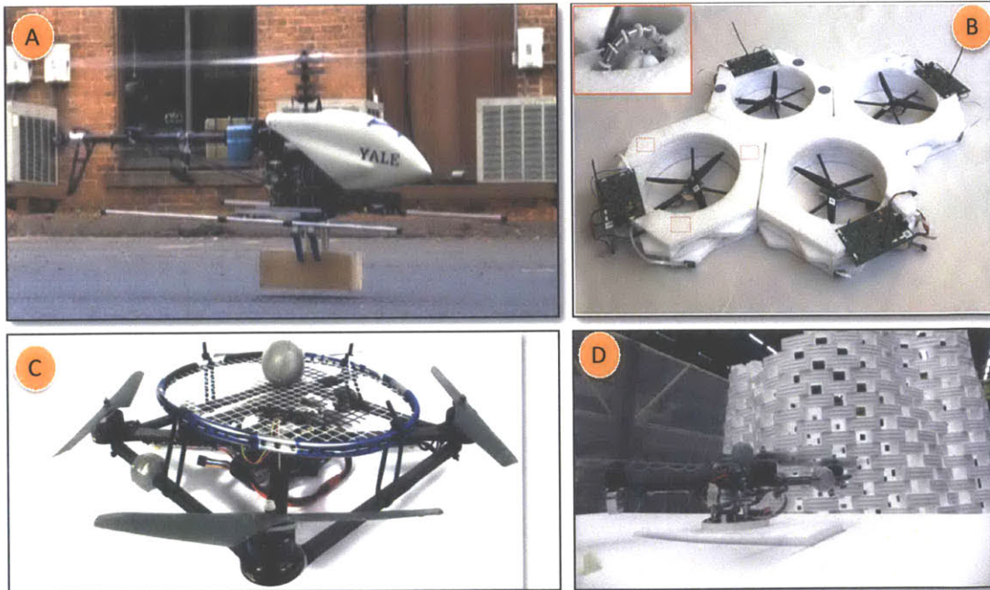
Figure 1.6: AAV based manipulation carried out at GRASP Lab of UPenn [12, 13, 19-21]. (A) Three Quadrotors cooperatively carry a payload using cables as the interface. (B) A Quadrotor is equipped with a gripper that can grasp an object. (C) Using gripper, the Quadrotor assembles the individual pieces to form a structure.
