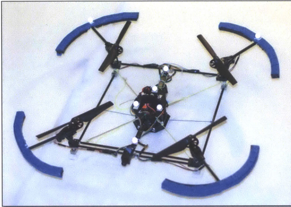
Figure 6.5: Version 2 of ParaFlex showing the protective shrouds around the propellers.
