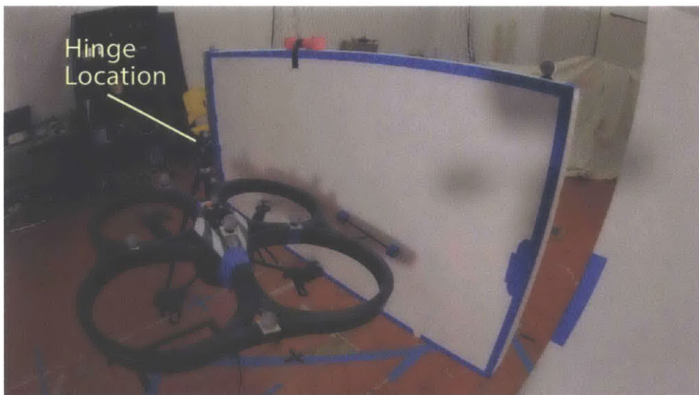
Figure 5.12: Another view of the experiment showing Quadrotor along with the end-effector docked to the door.
