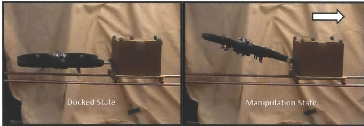
Figure 4.11: The Quadrotor is docked (left) and is pushing the cart (right) by making \theta > 0 .
