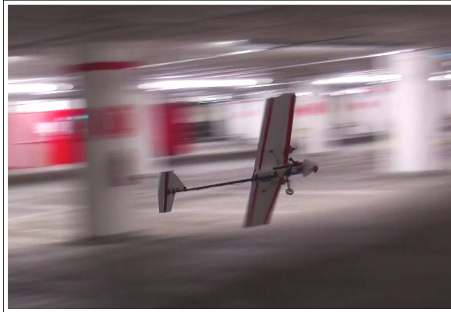
Figure 1-1: A picture of the robust robotics group's autonomous fixed wing aircraft flying in a parking garage area. During the flight depicted the vehicle had access to a prior map of the environment. This thesis seeks to develop algorithms that could enable the vehicle to not require a map ahead of time.
