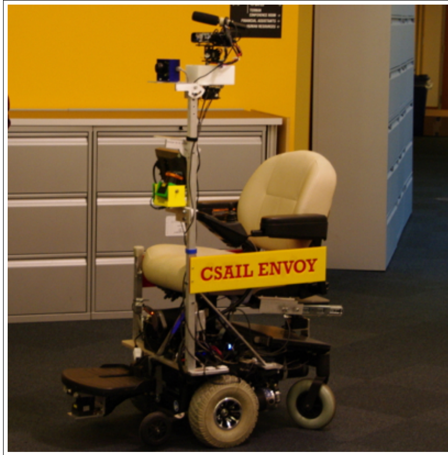
Figure 7-1: A picture of the robust robotics group’s autonomous wheelchair. The vehicle is outfitted with a number of sensors including cameras and lidars that we use to collect data.
