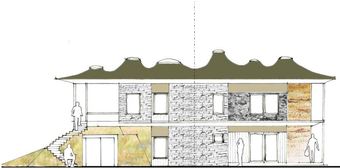
Elevation: Rear Back-Yard Side, Showing Exterior Private Entry to Second Floor
