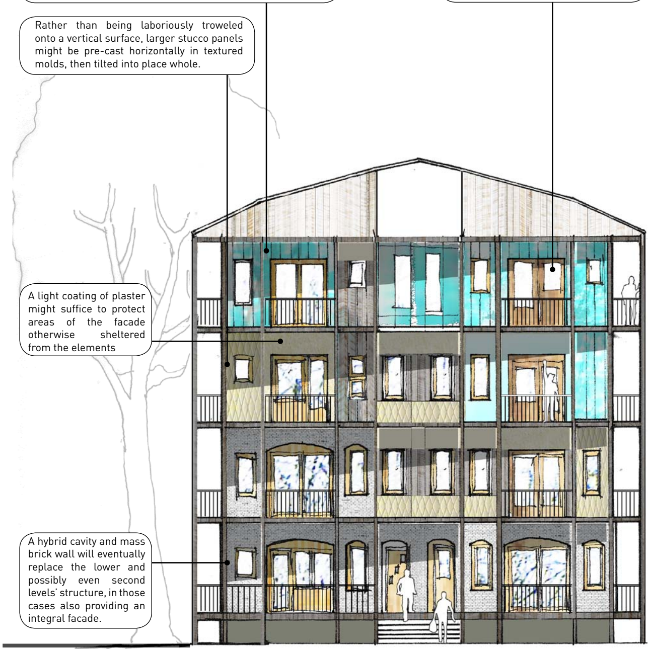
Street-Front Elevation: Conjoined Adjacent Parcels Showing Articulated Facade Under Construction
