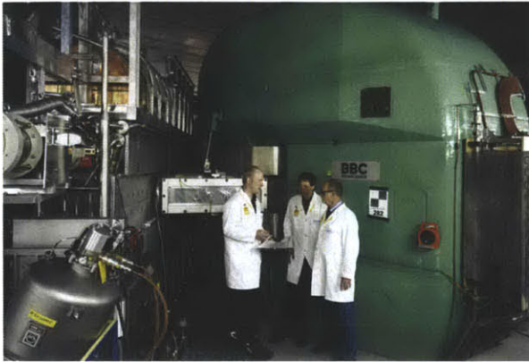
Figure 1.4 – 5.6 meter tall isochronous cyclotron located at the Paul Scherrer Institute
