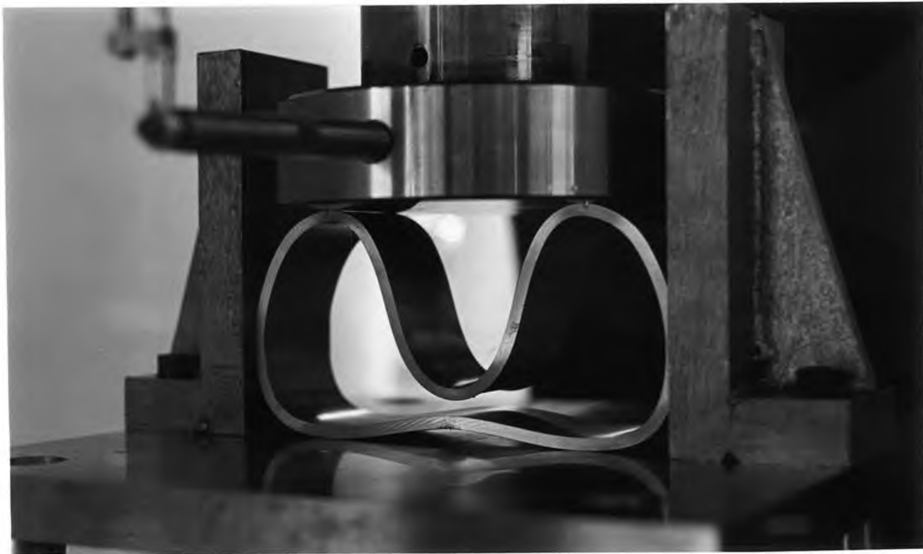
Figure(67)The deformation of a ring between two rigid parallel surfaces and two lateral walls with an initial gap
