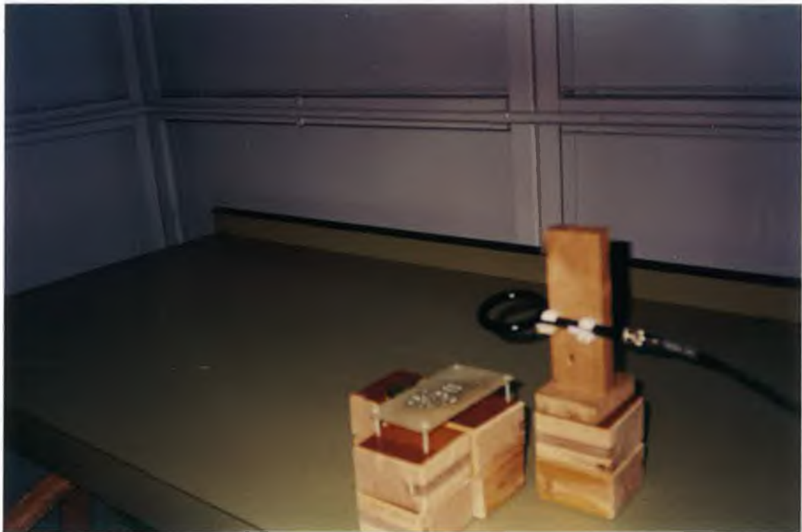
Fig. 7.4 Photograph of the near magnetic field measurement set-up.
