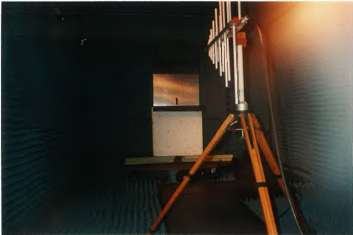
Fig. 6.9 Photograph showing the relative positioning of the Q-loop antenna and the LPA for vertical polarization mode.
