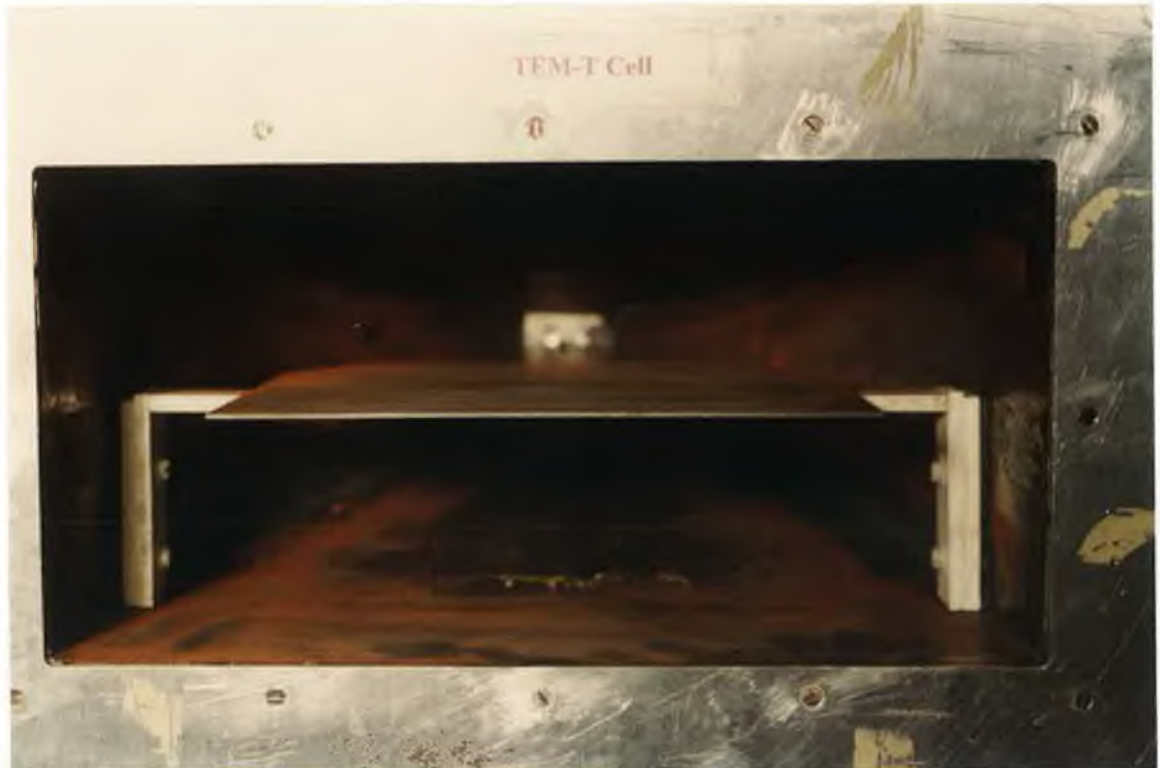
Fig. 4.8 Photograph of one half of the TEM-T cell (looking into the cell). Septum and dielectric support is shown in the diagram.
