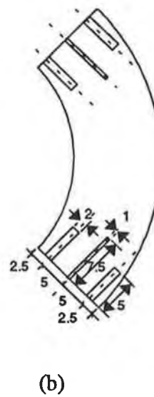
Fig. 4.15 Detail design of the Quarter of a loop. The screw positions for end connections and hole for penetrating the centre stud of the panel jack have also shown (a) Isometric view (b) Sectional view. Dimensions along the width and depth are exaggerated for better understanding. All the dimensions are in mm.
