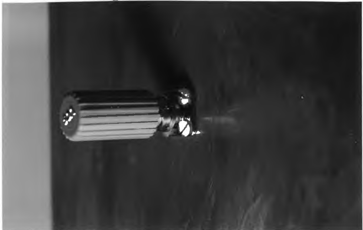
Fig. 4.14 Photograph of the rear end of the Q-loop antenna showing the end connections.
