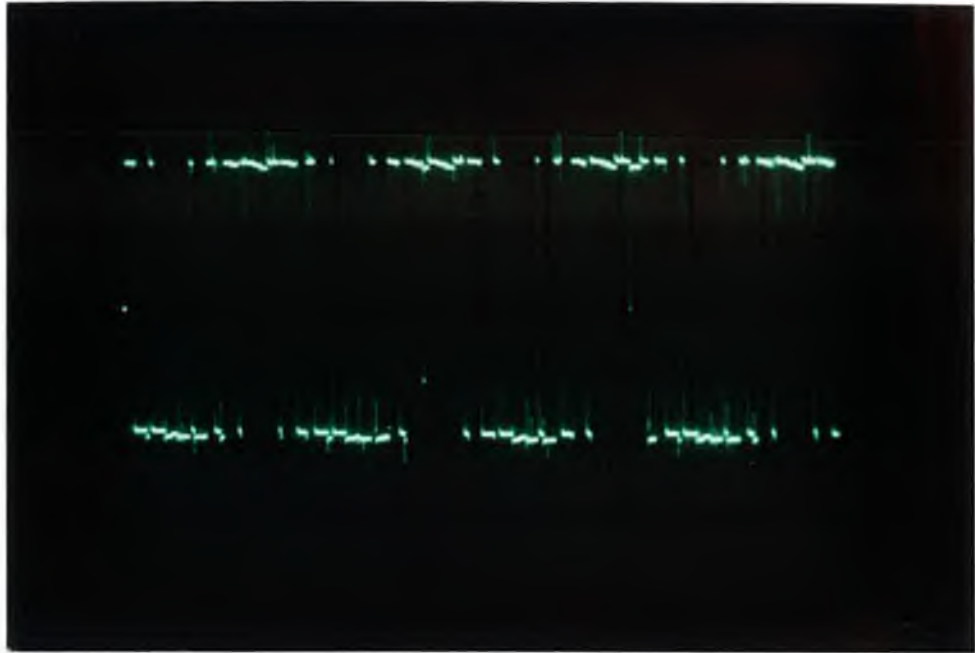
Fig. 7.1 Inverter output voltage (phase "A") 20 V/div Timebase = 1 msec/div
