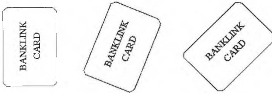
Figure 4.9 The three different positions each item was placed under the camera to extract colour information to compare with the database.
