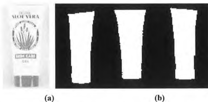
Figure 5.21 (a) Aloe vera container and (b) three different silhouettes obtained for the aloe vera container.
