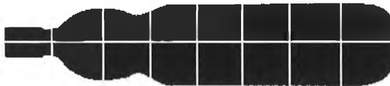
Figure 3.9 Diagram showing a bottle divided into eight sections using the rectangular coding method.
