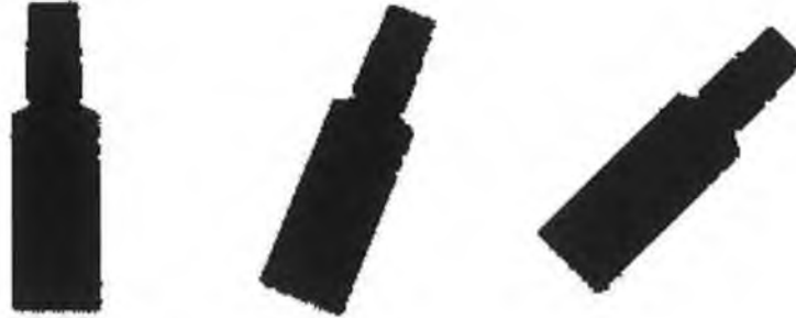
Figure 4.6 The three positions which each item was placed under the camera to obtain shape information to be compared with previous results.
