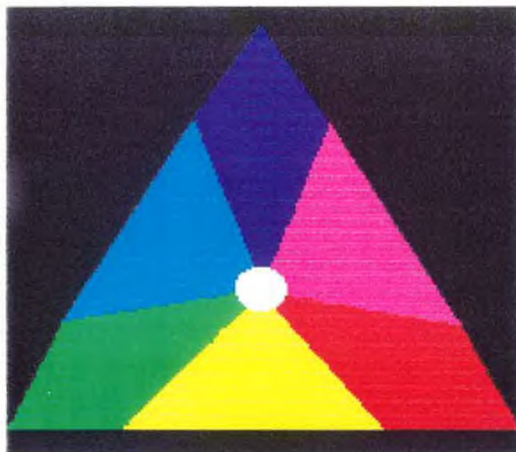
Figure 4.3 Colour triangle used to program the colour filter in the intelligent colour camera.
