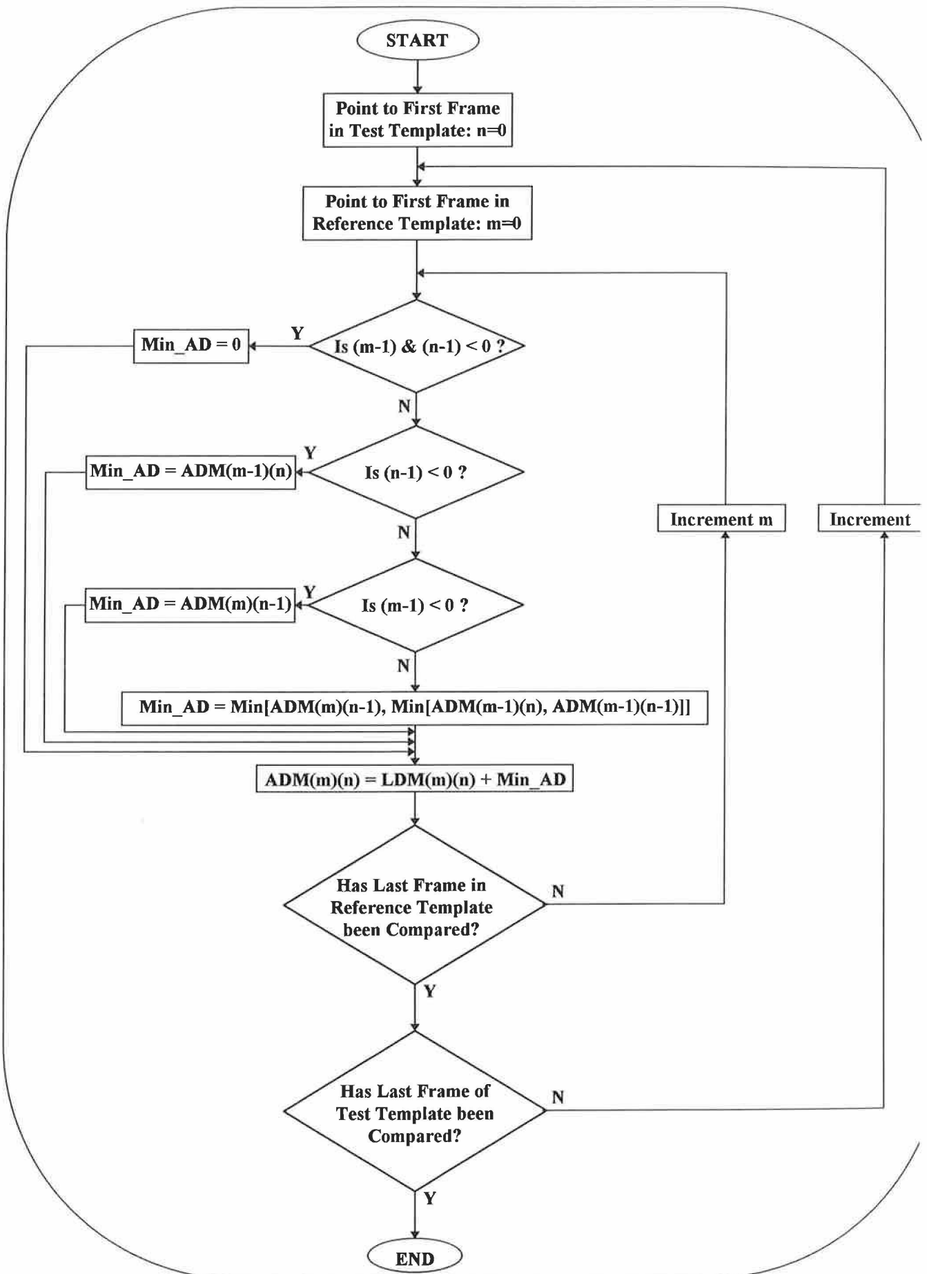
Figure 5.10: Flowchart describing the calculation of the Accumulated Distance Matrix (ADM) in DTW.
