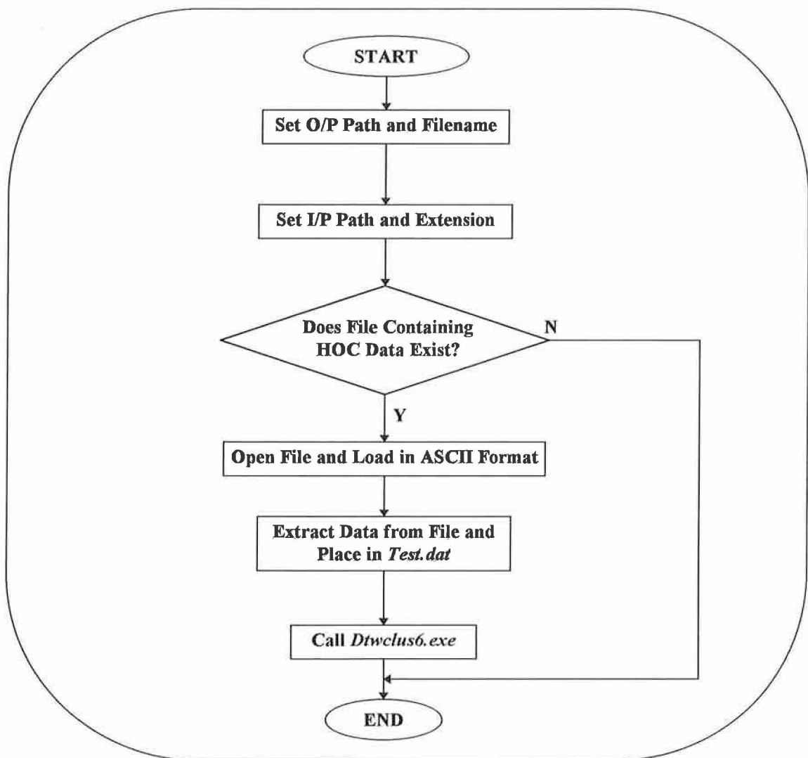
Figure 5.7: Flowchart explaining how Wordrec.m formats the CHOC data before recognition.
