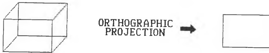
Figure 3.3: Orthographic projection of a cube
