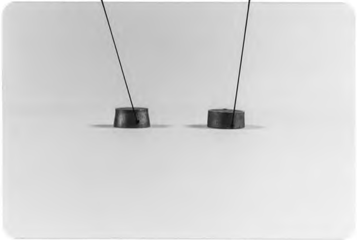
PLATE NO [3.6] EFFECT OF THE FRICTION ON THE FINAL SHAPE OF THE DEFORMED TEST SPECIMEN.
