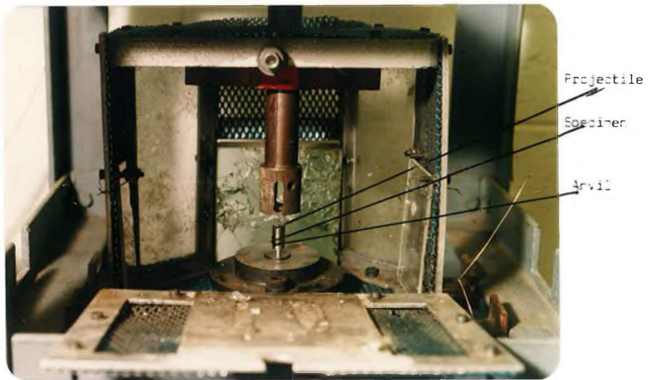
PLATE(3.5) Fire the Projectile against the test specimen placed in rigid anvil.
