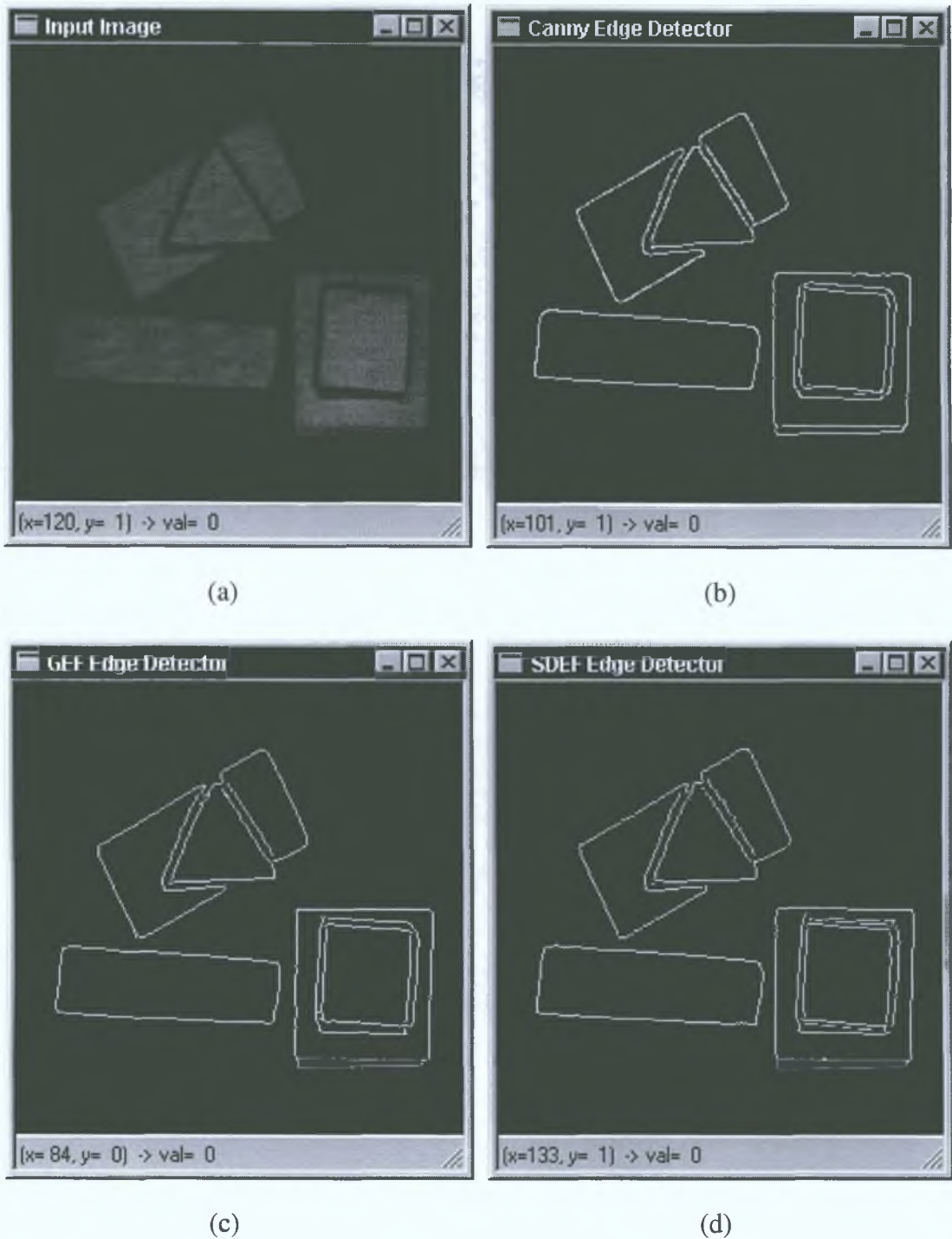
Figure 3.27. Edge estimation when the input is a raw image. (a) The input image. (b) The output from the Canny edge detector ( \sigma = 1.0 ). (c) The output from the GEF edge detector ( a_0 = 0.45 ). (d) The output from the SDEF edge detector ( a_0 = 0.55 ).
