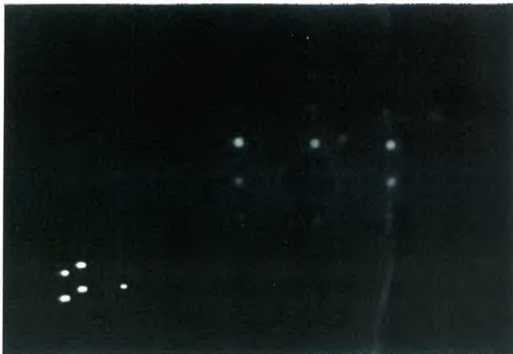
Fig 5.15 The S/GaAs(100) - (2x1) LEED pattern formed after annealing above 350°C
