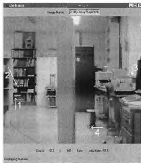
Figure 5-61. Displays a frame from the laboratory 2 image sequence at a threshold of 25. There are 4 more corners detected by the original SUSAN corner detector and these are shown here.
