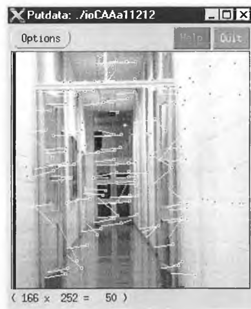
Figure 4-2. The extracted motion vectors using the developed algorithm.
