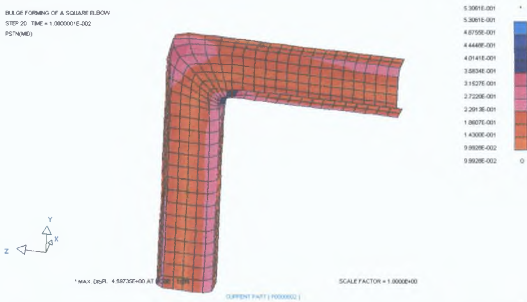
Figure 4.215: Distribution of plastic strain in the mid-plane of the elbow formed keeping the ends fixed
