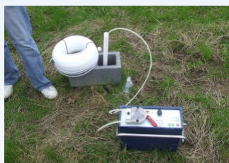
Plate 1: The collection of subsurface water from a monitoring well.
