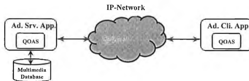
Figure 3-7 QOAS deployment at the level of an adaptive client-server system
