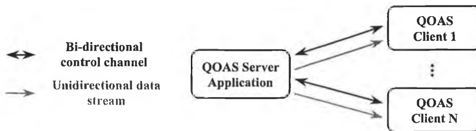
Figure 4-17 Multimedia data transmission and control data exchange between QOAS server and client applications
