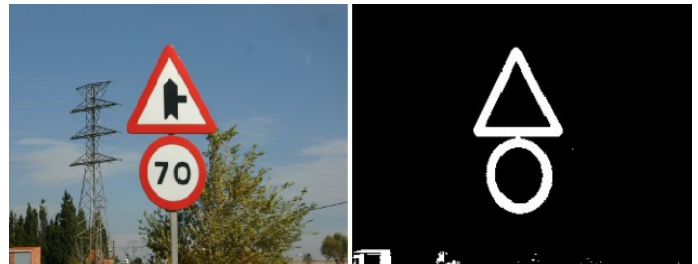
Fig. 2. An example illustrating the red color segmentation for two mutually occluding traffic signs that are attached to the same pole.
