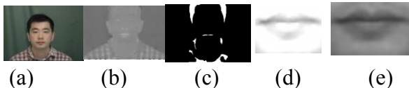
(a) RGB image. (b) Pseudo-hue image. (c) Image resulting after the application of the histogram-based thresholding. (d) Lips region – pseudo hue. (e) Lips region – gray-scale.
