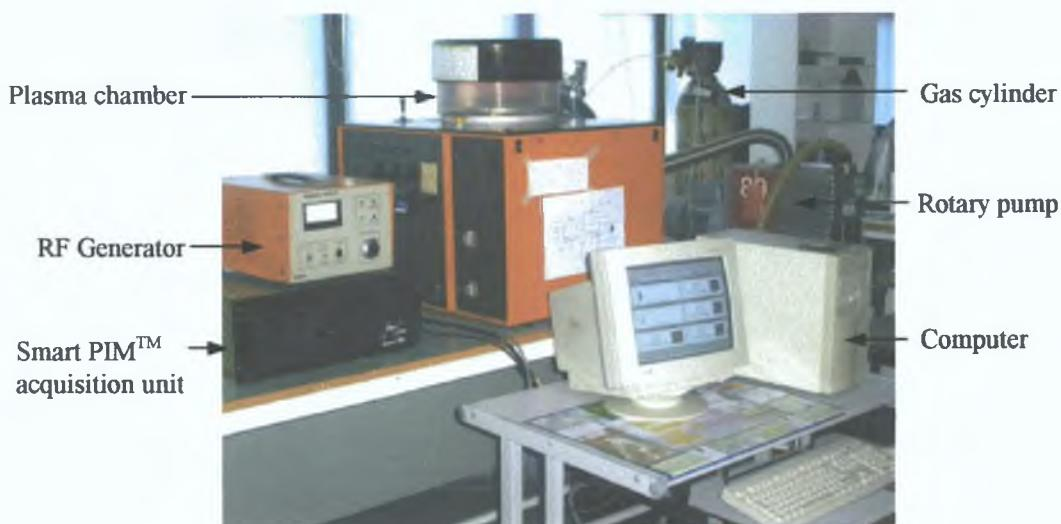
*Figure A.1* Capacitively driven, parallel plate, RIE system with the Plasma Impedance Monitoring monitor.
