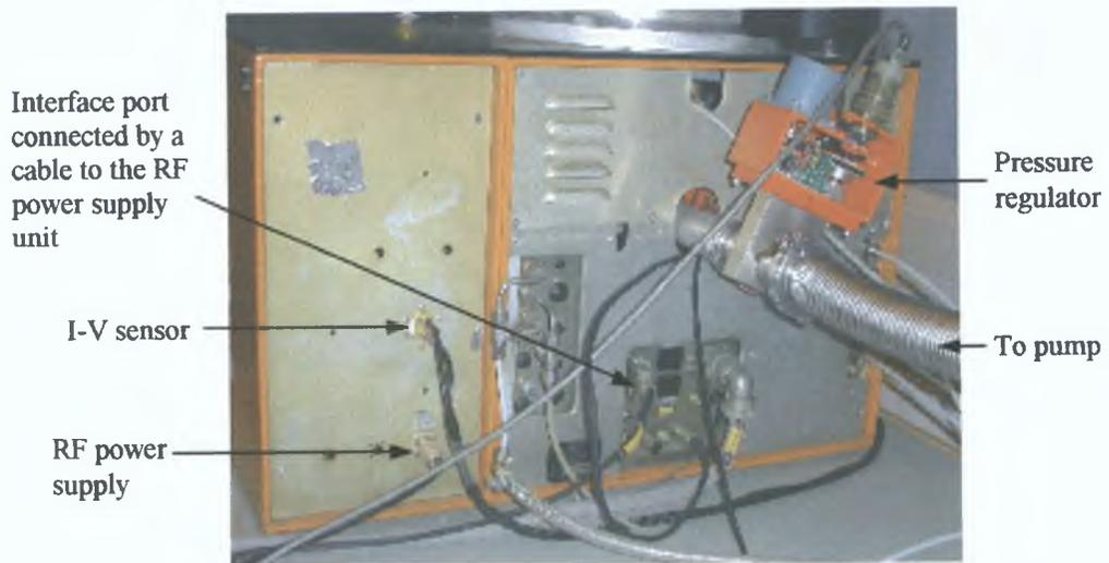
*Figure A.3 Back panel of the main RIE equipment.*
