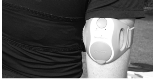
Figure 2.5 A biometric devices as worn by a user – the BodyMedia Armband is fitted to the arm.
