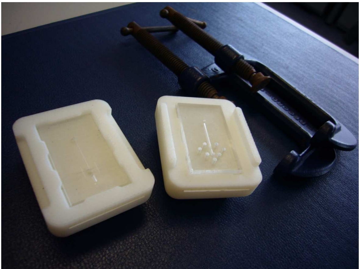
Figure 3.9: Assembly of Lab-on-a-Chip in 3D printed jig
