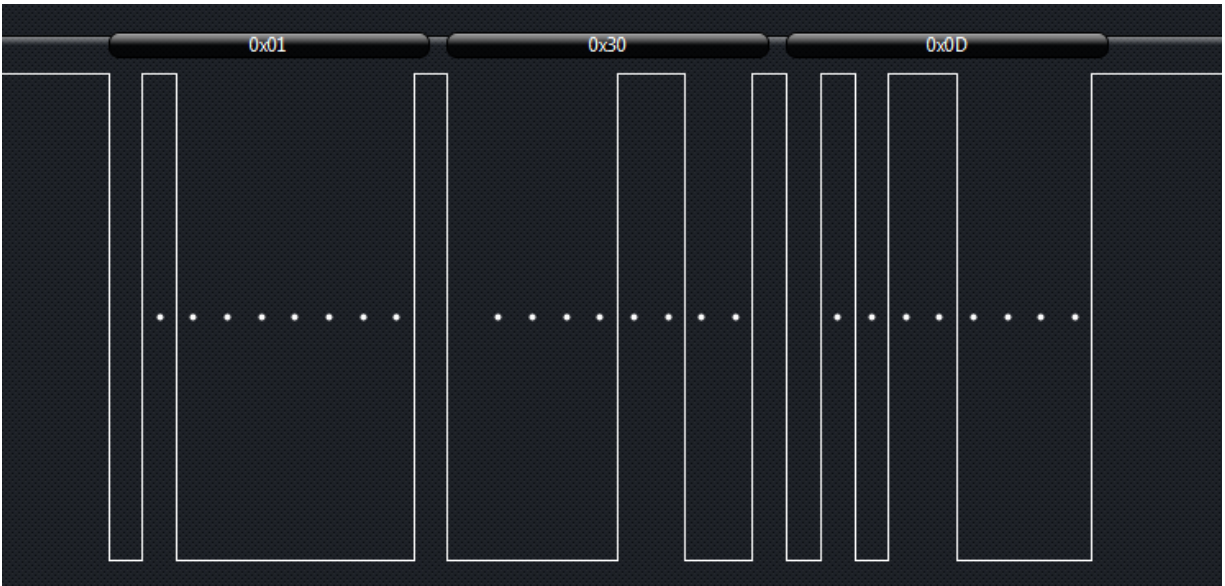
Figure 9: UART 8-N-1 3-Byte Data
