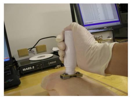
Figure 37. Experiment on a UHF system: knee implant wrapped by pig skin
