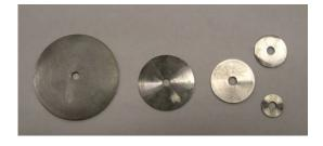
Figure 9. Round electrodes with variable sizes
