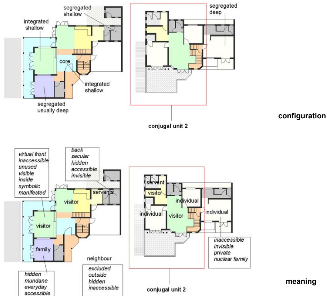
Figure 10: Configuration and meanings of a typical M model house ( Source: Authors)
