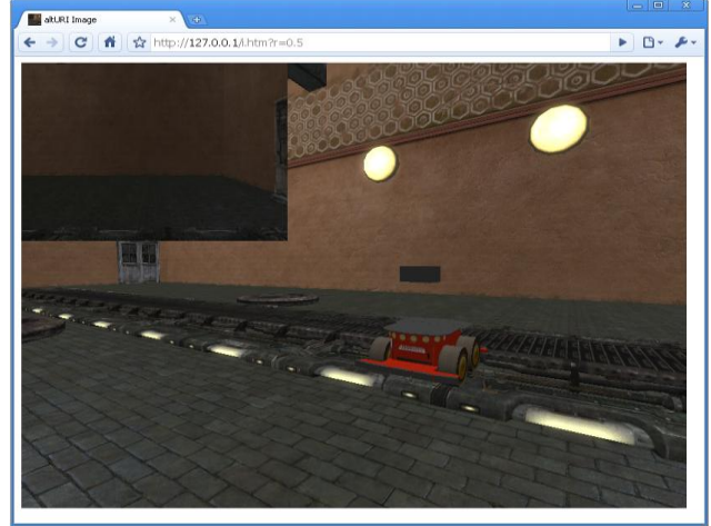
Figure 6. Google Chrome Browser showing 800x600 pixel image, 'movie' refreshing twice every second: USARSim UT3 Conveyor map with P3AT Robot.
