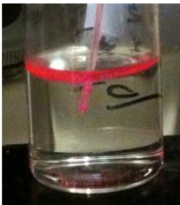
Figure 27. Collection and separation of the droplets from the biphasic flow. Bigger oil droplets floated and the smaller double emulsion droplets with less of the pink dye sank in the bottom of the collection vial.
