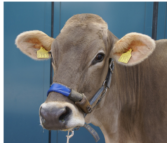
Figure 1 Cow with recording halter. Cow fitted with a recording halter incorporating an oil-filled tube and pressure sensor. The brown leather pouch near the cheek band contains the data logger.
