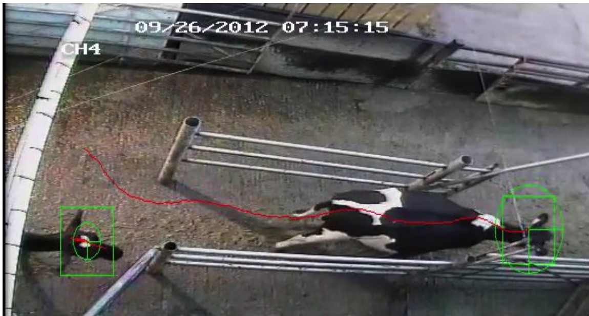
Figure 2: Detected and tracked cows. Green squares show the location of detected heads; green circles show the Kalman filter uncertainty in the true location and red lines indicate the true path followed and can be used to measure gait asymmetry.
