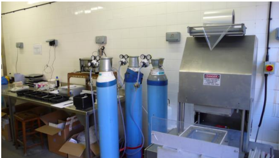
Figure 3.3. Image showing the MAP machine with the gas cylinders used in the MAP trials.
