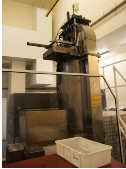
Figure 4.12 Image showing the high-pressure machine at the Northern Ireland Agri-Food and Biosciences Institute used in the high hydrostatic pressure experiment.
