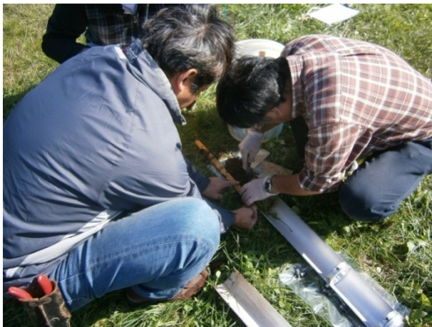
Cutting a core into depth sections
