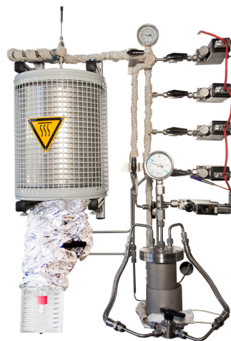
Figure 6.5.: Flow setup with heated tubes before and after the reactor.
