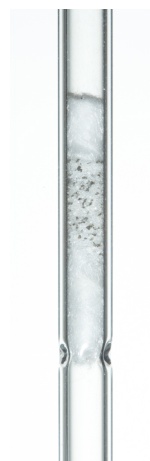
Figure 3.3.: Quartz reactor with a loaded sample fixed between two layers of quartz wool and diluted in \text{SiO}_2 .
