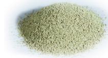
Figure 3.5.: Crushed and fractionated sample, where all the SiO_2 fibres have been removed.
