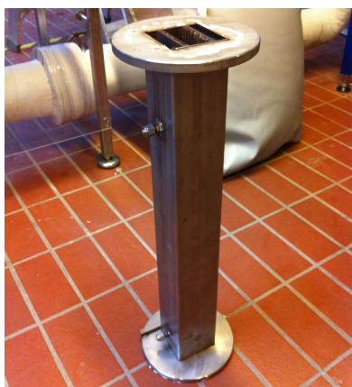
Figure B.8.: (Left) reactor without heating element and with cassette for catalyst plates. (Right) particle distribution of potassium aerosols.
