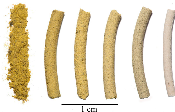
Figure 5.4.: Extrudates made using the optimised 20 wt.% V_2O_5/TiO_2 catalyst and 0, 10, 20, 30, 50 wt.% and pure sepiolite (from the left).
