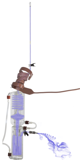
Figure 6.3.: Column for SO 3 absorption, heated to 80 °C by flowing water to avoid H 2 O condensation.
