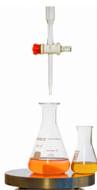
Figure 6.4.: Titration of SO 3 containing washing solution of H 2 O/iso-propanole with Barium perchlorate and a Thorin indicator.
