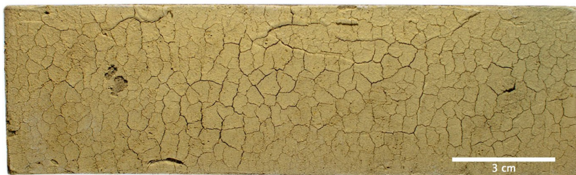
Figure B.10.: Composite plate catalyst comprising a \text{SiO}_2 mesh and a 20 wt.% sepiolite / \text{V}_2\text{O}_5/\text{TiO}_2 mixture.
